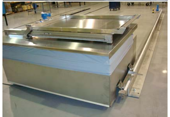
Clockwise from above: the Portable Cart from a semi-automatic system; vials loaded onto the automatic guided vehicle (AGV) shelf; the AGV seated on the X-Rails.
